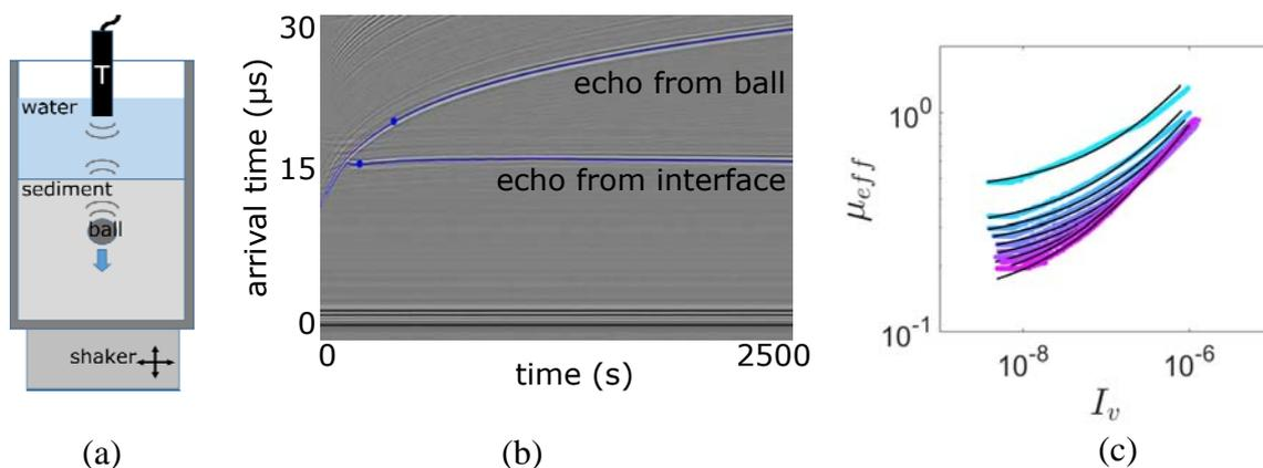
**Figure 1.** (a) Schematic of ultrasonic monitoring of a sinking ball in dense granular suspension, using a piezoelectric transducer (T). (b) Stack of waveforms showing the reflection of the sinking ball and of the interface. (c) Effective friction coefficient as a function of a viscous number  $I_v$  [2] for different vibrational intensities. The black lines represent a fit of the frictional rheology model.
