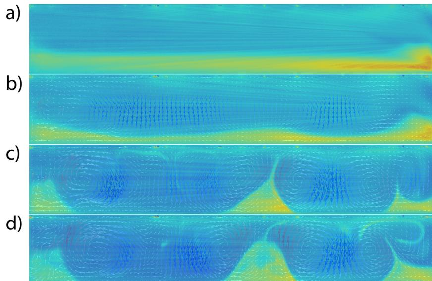
**Figure 1.** Cross-section of the experimental tank containing the optical image superposed on the 2D velocity field a) initial, stable condition, b) initiation of convection into the top layer, c,d) pile formation and tendrils entrainment.
