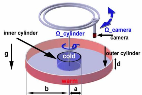
**Figure 2.** Sketch of the new experimental apparatus. The radius  $a$  ( $b$ ) of the inner (outer) cylinder is 12cm (70cm),  $d=30$ cm. Also visible is the feature tracking system that consists of a camera that can follow flow features due to the fact that the camera can rotate with a different angular velocity than the confinement. This setup is ideal to follow a baroclinic jet that usually rotates somewhat faster than the annulus.
