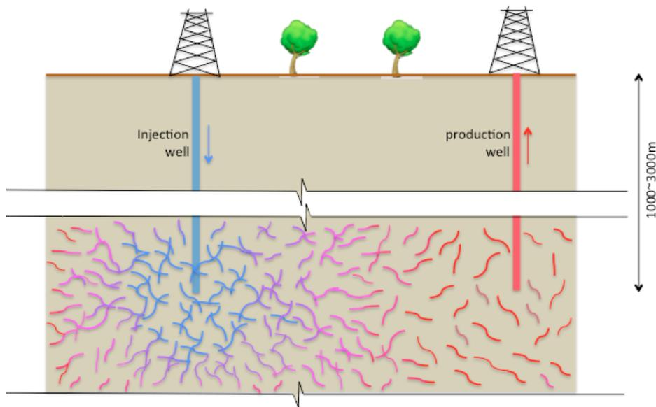
**Figure 1.** schematic of the stimulation process between a pair of geothermal wells.
