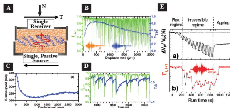
**Figure 1.** (A) Shear apparatus (B) Evolution of the shear with slip (in blue) and the cross-correlation of Coda waves shown inset (in green) (C) Monitoring the decrease of shear wave speed (D) Zoom into Fig. B. (E) Sound-induced fluidization in granular media.
