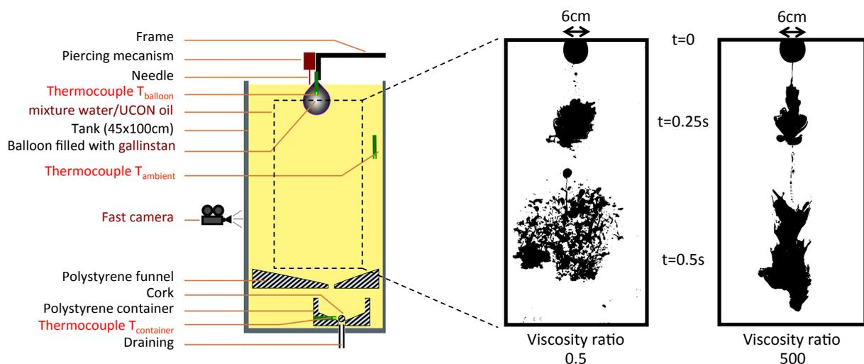
**Figure 1.** Sketch of the experimental set-up (left) and two examples of the observed sedimentation and fragmentation processes for identical initial metal blobs (right). Only the viscosity of the ambient fluid is changed between the two experiments, with pure water on the left and a mixture of water and Ucon oil on the right, leading to a viscosity ratio of 0.5 and 500 respectively. Each picture shows the liquid metal blob at two times following the balloon piercing at  $t = 0$ .
