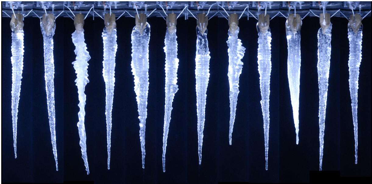
**Figure 1.** A selection of laboratory grown icicles with various morphologies. All of the data from this experiment is available online in the **Icicle Atlas**, [http://www.physics.utoronto.ca/Icicle\\_Atlas](http://www.physics.utoronto.ca/Icicle_Atlas).
