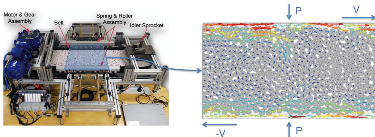
**Figure 1.** Granular vortices in experimental sheared granular flows. (1) Stadium Shear Device (SSD) where 2D grains are sheared within a belt; (2) Snapshot of the velocity of individual grains in the central section of the SSD showing the formation of granular vortices ( $V$  is the belt velocity and  $P$  the applied normal stress).
