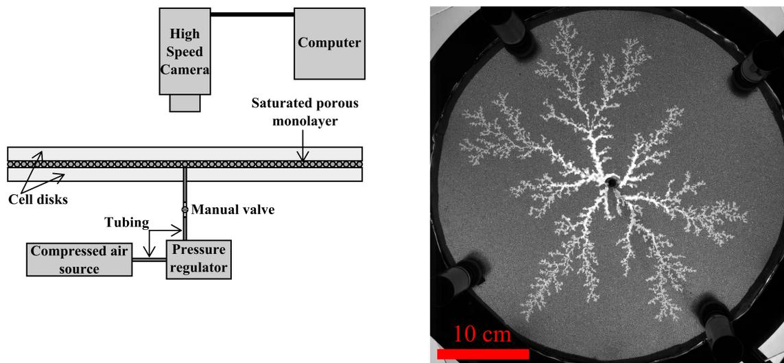
**Figure 1.** Sketch of our experimental setup seen from the side (left), and a top-down image at the breakthrough time of an experiment (right). During the experiment, air invades the saturated porous medium from the center, forms viscous fingers and induces deformations in the surrounding medium.
